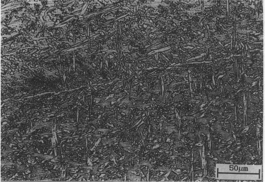
FIG. 7. Spatial organization of \alpha and \beta phases in a rod extruded from CuZn39Pb2 ingot at temperature 820°C on a press with reversibly rotating die.
