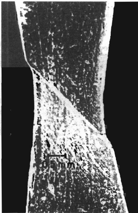
FIG. 4. Single crystal of aluminum - 2.8 wt. percent copper deformed in tension (after LISIECKI et al. [35]).
