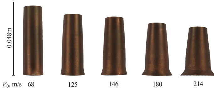
FIG. 7. Specimens recovered after the Taylor DIE.
